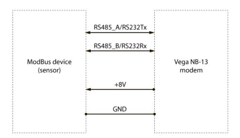
The modem can power up the ModBus device connected to it before polling it, for this use the "+8V" contact.
