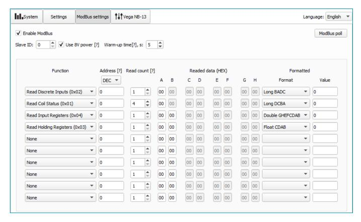
**Enable ModBus** – activates the ModBus functionality. The modem additionally polls the ModBus device by events and puts the received data into a black box. When sending to the server, the "modbus" key with data is added to the JSON message. If the checkbox is off, the ModBus device is not polled, therefore, ModBus data is not accumulated in the black box, the "modbus" key is missing in the JSON message.
