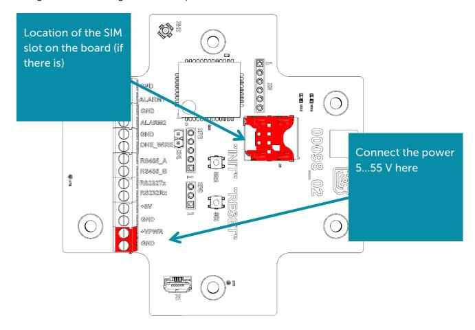
Vega NB-13 modem operate from the external power supply. In "Data collection" mode after power supplying the device loading and sleeps until the communication session according with the schedule.
